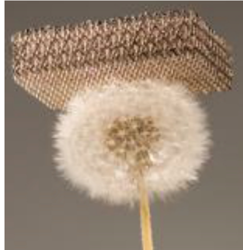
Fig. 1. An example of a 3D lattice structure, designed and fabricated by Hughes Research Labs (HRL), representing the new frontiers for materials and design. 99.99% of this metallic truss structure is air. The remaining 0.01% is made of very thin (nanometer, micron and millimeter scale) features.
