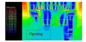
Fig. 10. summertime wind speed levels -teaching building 31 with opening in building shape.
