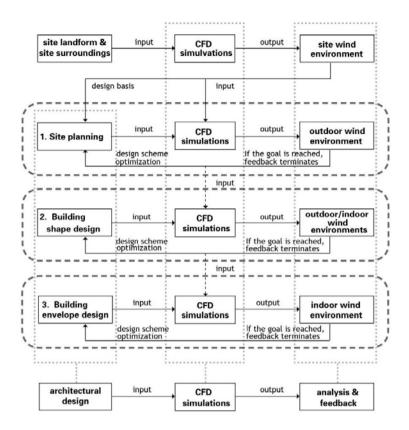
Fig. 15. flow diagram for optimized design of green building natural ventilation based on CFD simulation.
