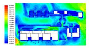
Fig. 14. wind speed levels at level 1.5m in rooms on F1 after final optimization.
