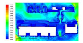
Fig. 11. wind speed levels at level 1.5m in rooms on F1 in preliminary simulation.
