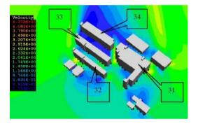
Fig. 7. summertime wind speed levels - no open-up design.
