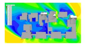
Fig. 4. wind speed levels - all corridors enclosed.
