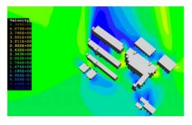
Fig. 8. summertime wind speed levels -teaching building 31-34 with partial open-up design.
