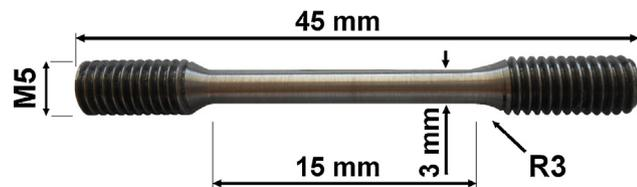
**Fig. 3 – View of a sample prepared for the uniaxial tensile test and its basic dimensions.**
