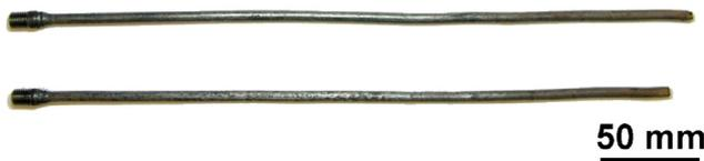
**Fig. 1 – View of bulk nc-Ti in the form of rods with a diameter of  $\varnothing 5$  mm.**
