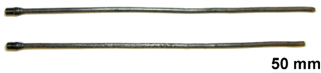
Fig. 1 – View of bulk nc-Ti in the form of rods with a diameter of \varnothing 5 mm.
