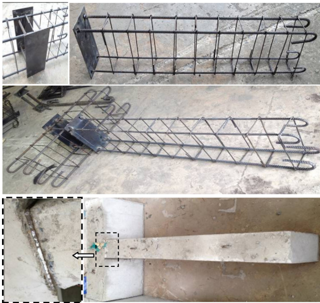
Fig. 2 – A set of the steel reinforcements, and reinforced concrete specimens with welded plate joint.
