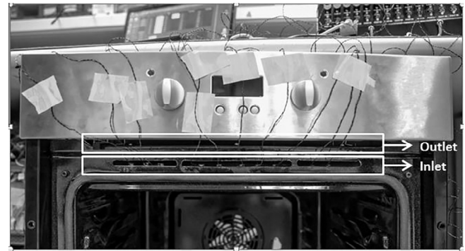
Fig. 4. Arrangement of anemometers in experimental study.
