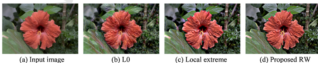
Fig. 12. Detail exaggeration using our tool. The detail enhanced results (3×). Parameters: L0 ( \lambda = 3E-2 ), local extreme (17), and proposed RW ( \mu = 0.005, \beta = 9 ).
