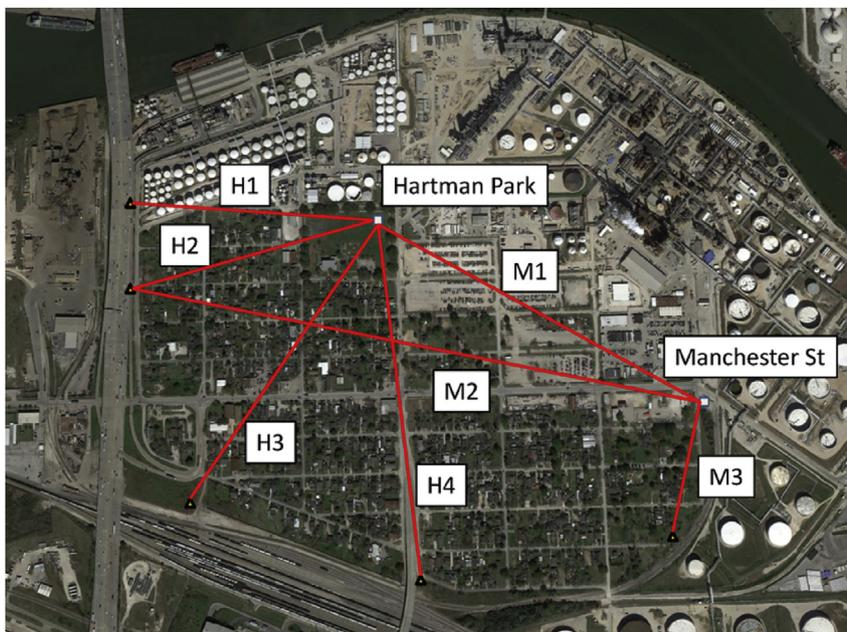
Fig. 9. Setup of the two LP-DOAS instruments and the seven light paths during the BEE-TEX experiment in the Manchester neighborhood in Houston, TX.
