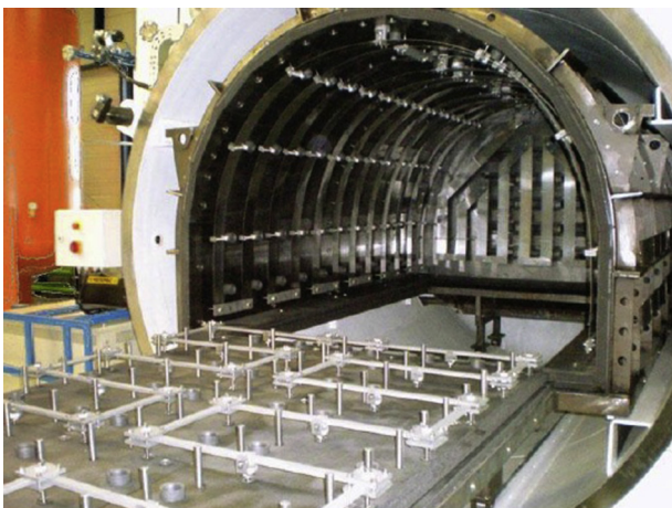
Fig. 1 – TWC INVAC-made high-vacuum furnace with removable bottom used for titanium brazing [6].
