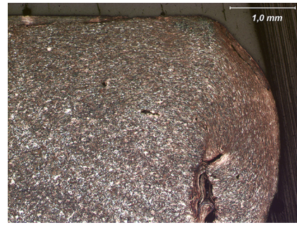
Fig. 6 – A microscopic image of the structural alterations and damages. Elongated visible (light) parts are ferrite separations. Magn. 25x, etched 3% HNO_3 , light microscopy.
