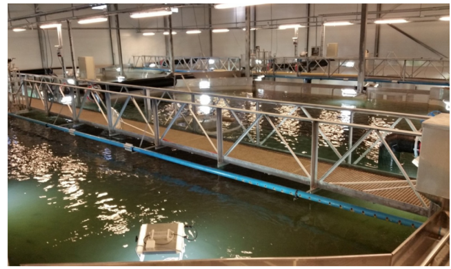
Fig. 1. Example of octagonal tanks (14.5 m wide × ~4 m deep) grouped together in one of the recirculating systems at the Marine Harvest Steinsvik hatchery.
