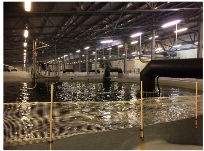
Fig. 2. Example of circular tanks (16 m diameter × 3.3 m deep) grouped together in one of the recirculating systems at the Grieg Seafood, Adamselv Culture Station.
