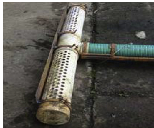
Fig. 3. Photograph of sludge sucker attached with sludge pump.
