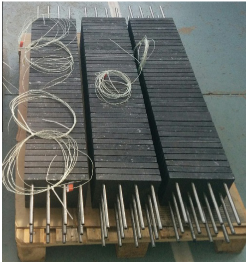
Fig. 8. Photo of the tube bundles through the composite plates.
