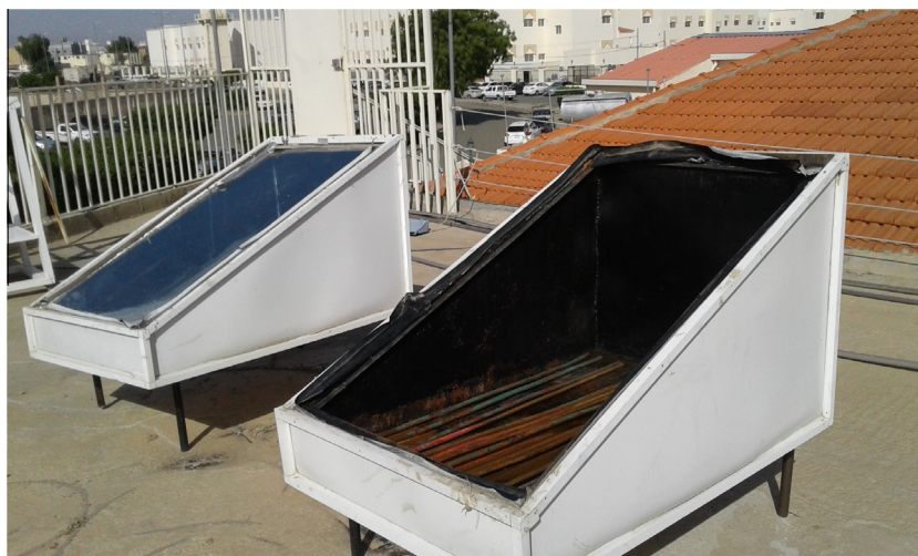
Fig. 1. Photographic view of a single type basin solar still with/without paraffin wax (PW).
