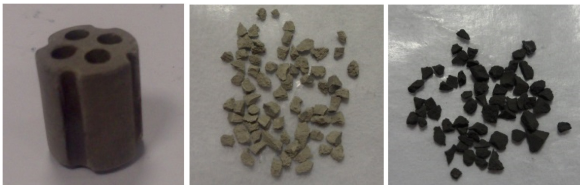
Fig. 1. Photos of catalyst pellet, fresh catalyst particles and reduced catalyst particles.
