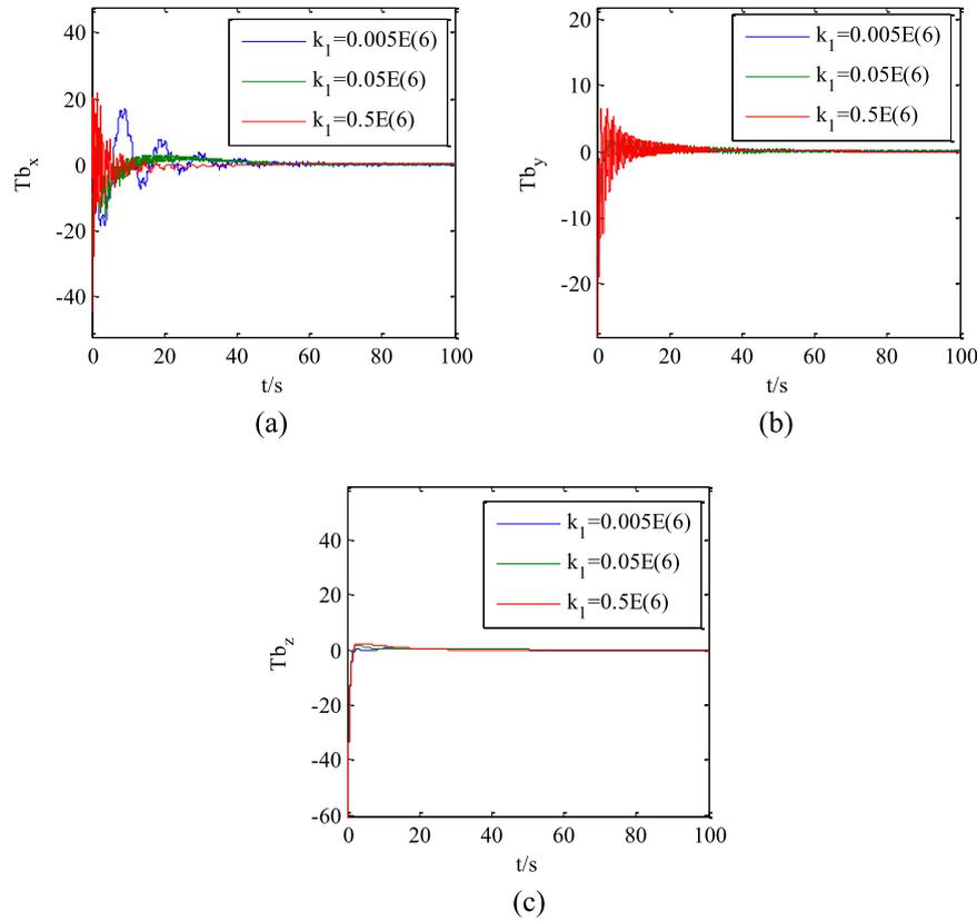
Fig. 5. Control torque of the flexible spacecraft.
