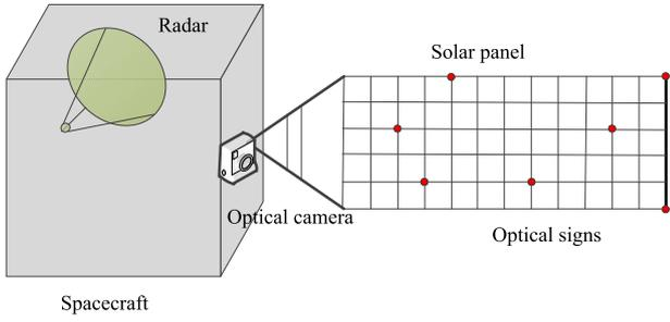
Fig. 1. Configuration of the flexible spacecraft.
