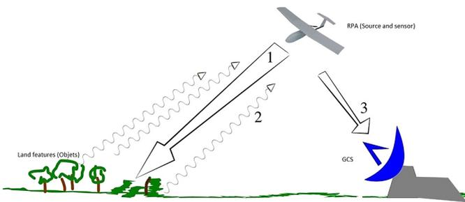
**Fig. 1.** Remote sensing using passive sensor system.
