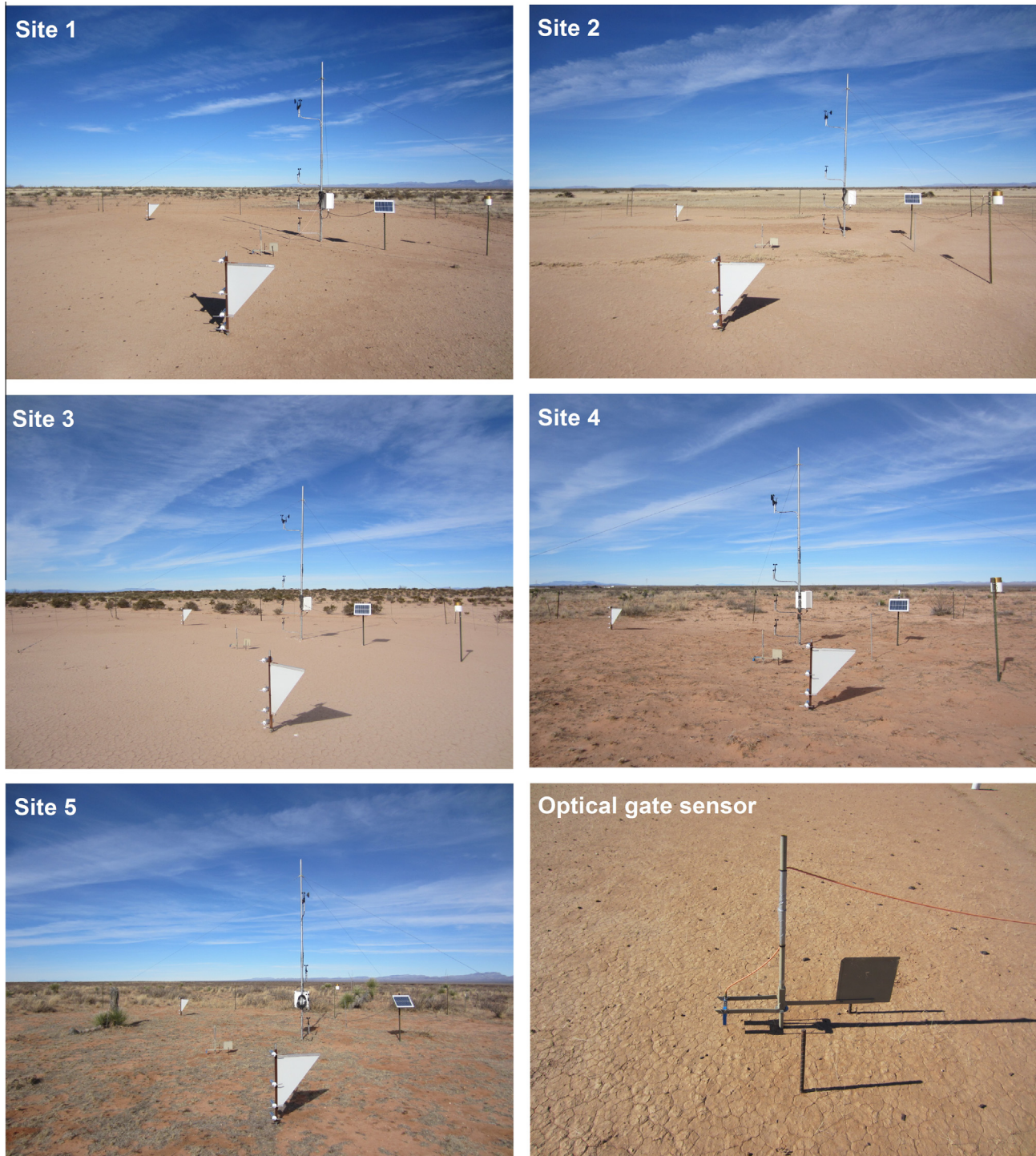
Fig. 2. Photographs of the five study sites showing meteorological towers, two MWAC sediment samplers and close-up view of a Wenglor optical gate sensor mounted on a wind vane. Stakes either side of the wind vane restrict the Wenglor rotation so that it samples within the range 180^{\circ} – 270^{\circ} . Photographs were taken from the south, facing north.
