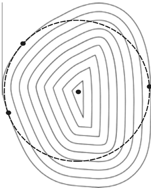
Fig. 6. Planar illustration of ventifact formation by uniform abrasion. The distances between adjacent curves are constant. Typically, initially rounded objects develop flat facets at initially flatter portions, and sharp vertices where the initial shape is more curved. The object shrinks to the internal point furthest from its external surface, which is the center of the largest inscribed circle in 2D or sphere in 3D (dashed lines). The shape of the solid becomes polygonal with as many edges as the number of tangencies of the circle (in this case 3). Three dimensional objects similarly develop facets, edges and vertices. The number of facets of a worn shape are determined by the number of tangencies of the inscribed sphere in the initial state.
