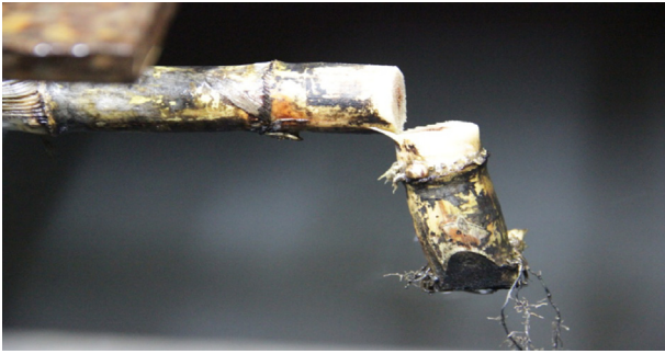
Fig. 7. Sugarcane cutting using a waterjet.
