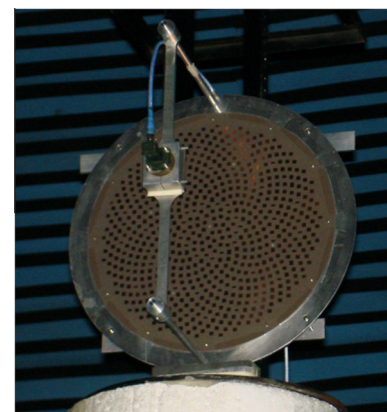
Fig. 6. Fabricated reflectarray along with feed horn.
