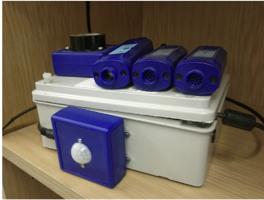
Fig. 2. Sensor box in situ , showing PIR, temperature, CO 2 , light, sound and humidity sensors.
