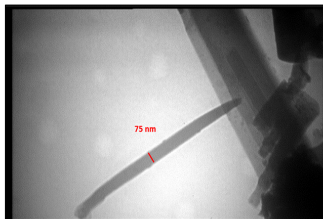
Fig. 2. TEM micrograph of the synthesized SA nanoparticles.
