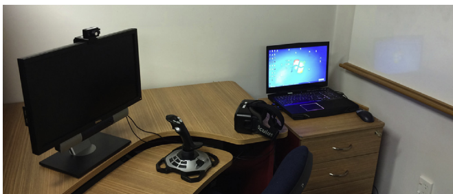
Fig. 3. Experiment components including monitor, joystick, HMD, laptop, and HMD tracker placed at the top of the screen.
