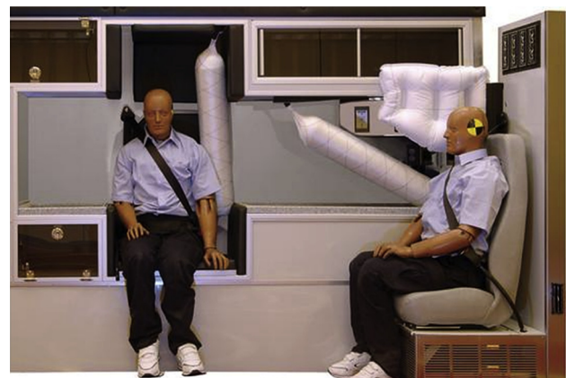
Fig. 3. Horton Ambulance airbag design.
