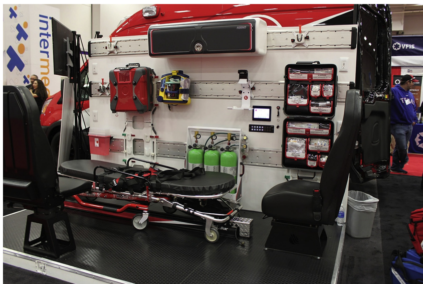
Fig. 5. Ferno modular rail system, presented at the 2015 EMS conference in Dallas.
