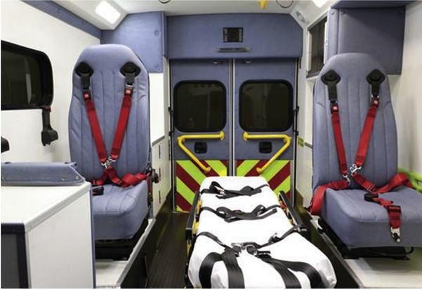
Fig. 4. MIT ambulance bench & seat reconfiguration (Forgues, 2014).
