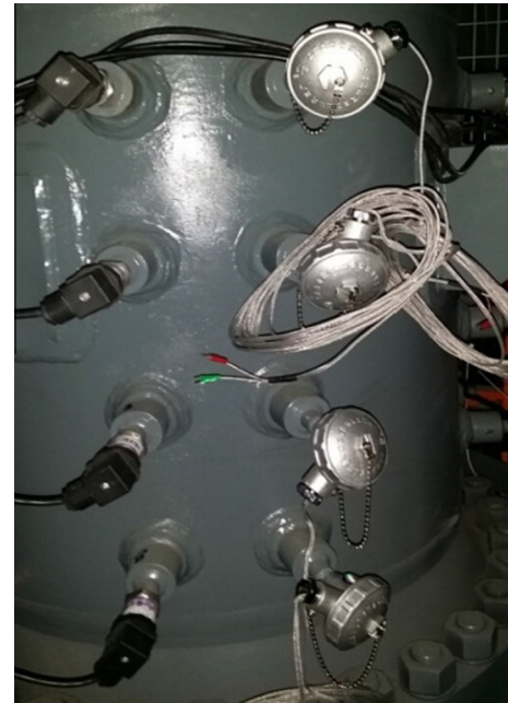
Fig. 3. Pressure vessel and measuring instrument.
