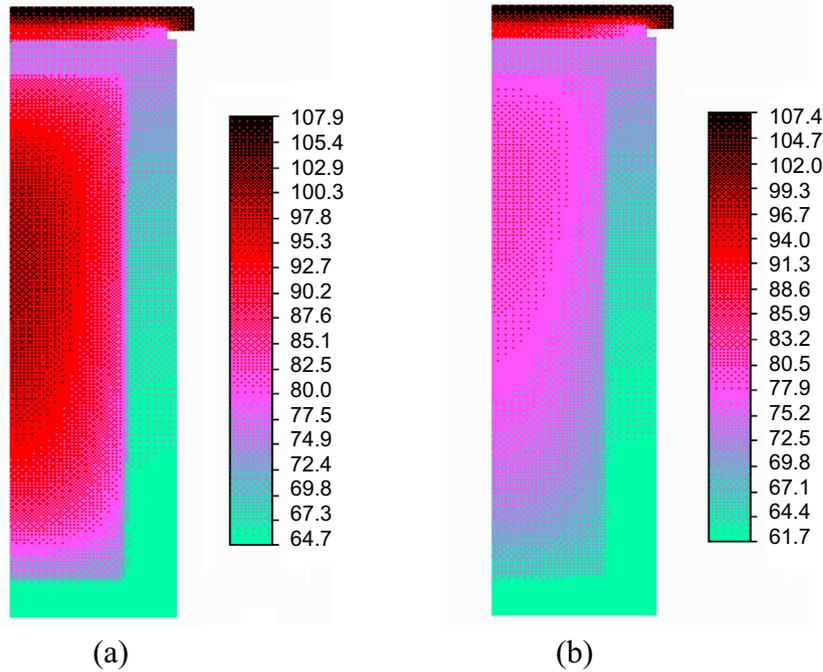
Fig. 4. Temperature distribution inside the cask and in the body of the cask in summer conditions: (a) after 100 years of storage and (b) after 300 years of storage.
