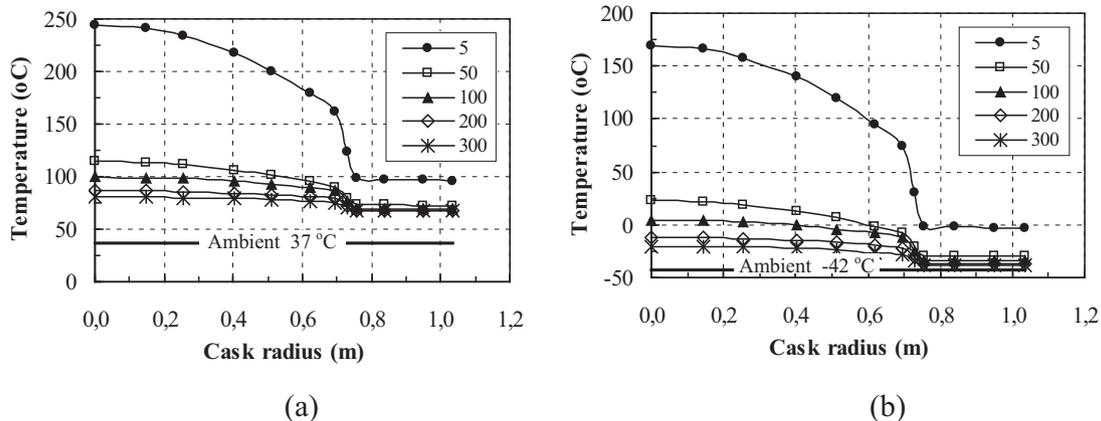
Fig. 6. Temperature distribution in the radial direction of the cask depending on storage time: (a) in summer conditions and (b) in winter conditions. 5 and 50 years – from Pořkas et al. (2006); 100, 200 and 300 years – this study.
