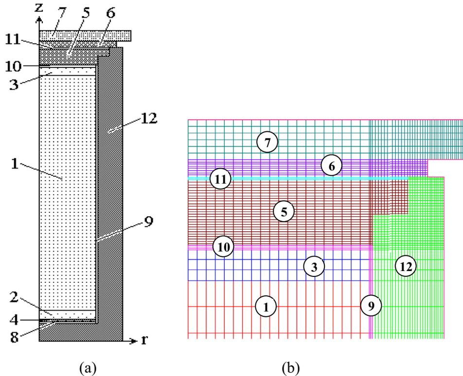
**Fig. 2.** Schemes of the cask computer model (a) and enlarged mesh (b): 1 – active fuel load part, 2, 3 – lower and upper fuel load parts, 4 – basket bottom, 5 – cask lid, 6 – guard plate, 7 – concrete cover, 8–10 – lower, vertical and upper He gaps, 11 – air gap, 12 – cask body.
