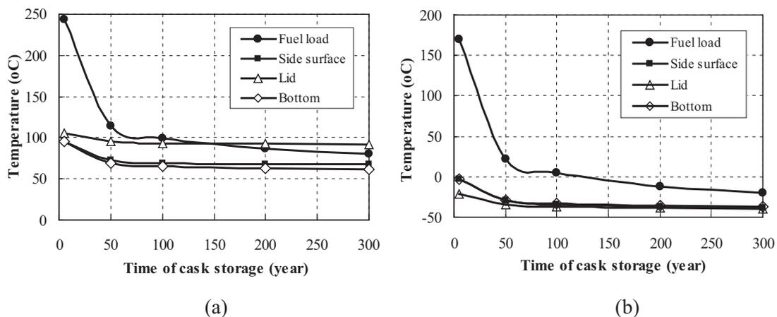
Fig. 7. Temperature variation with time in the characteristic locations: (a) in summer conditions and (b) in winter conditions.
