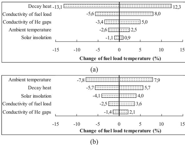
Fig. 8. Tornado diagrams for maximal fuel load temperatures in summer conditions: (a) after 5 years of storage and (b) after 100 years of storage.
