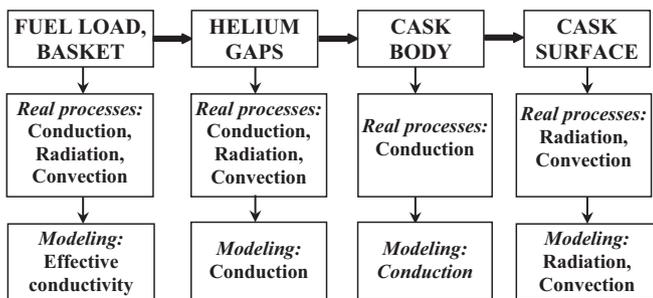
**Fig. 3.** Scheme of heat transfer through the cask.
