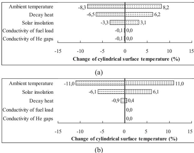
Fig. 9. Tornado diagrams for cylindrical surface temperatures in summer conditions: (a) after 5 years of storage and (b) after 100 years of storage.
