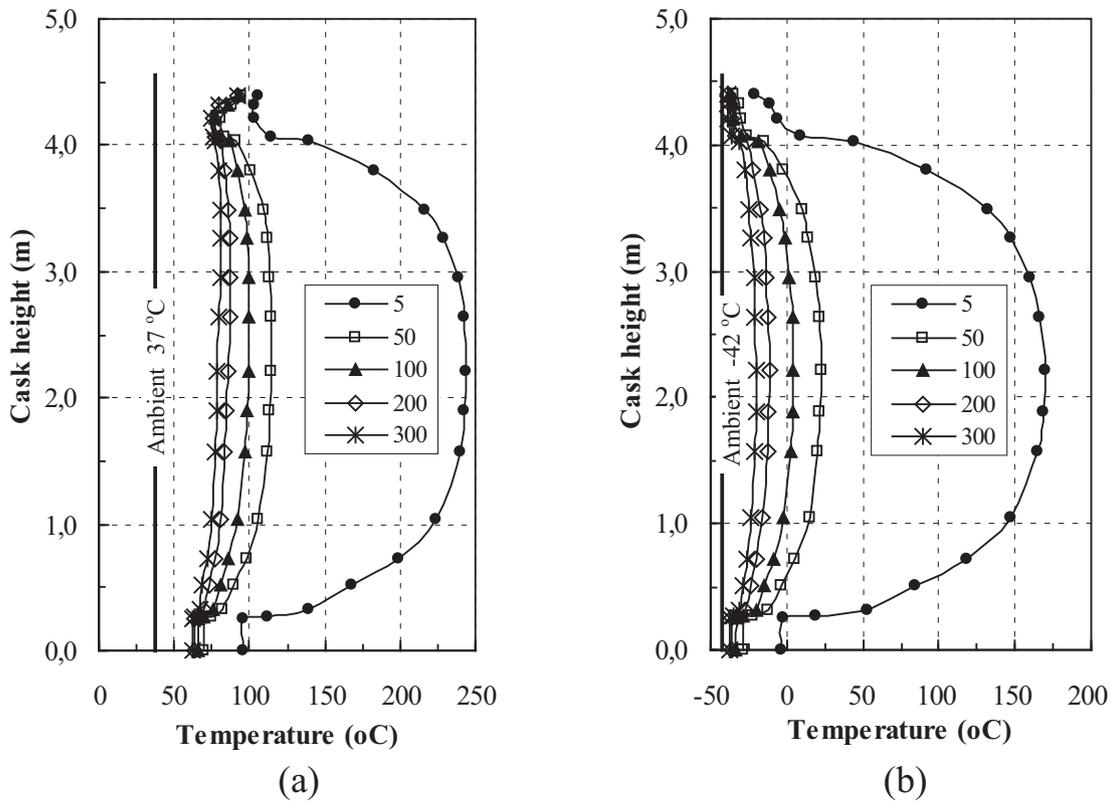
Fig. 5. Temperature distribution in the axial direction in the center of the cask depending on storage time: (a) in summer conditions and (b) in winter conditions. 5 and 50 years – from Pořkas et al. (2006); 100, 200 and 300 years – this study.
