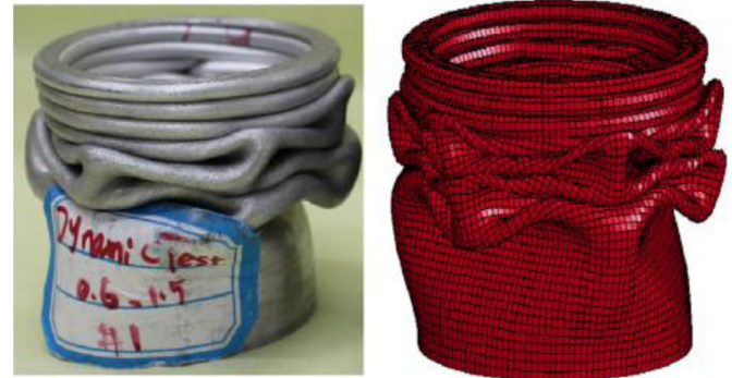
Fig. 5. Comparison of experiment and simulation model.
