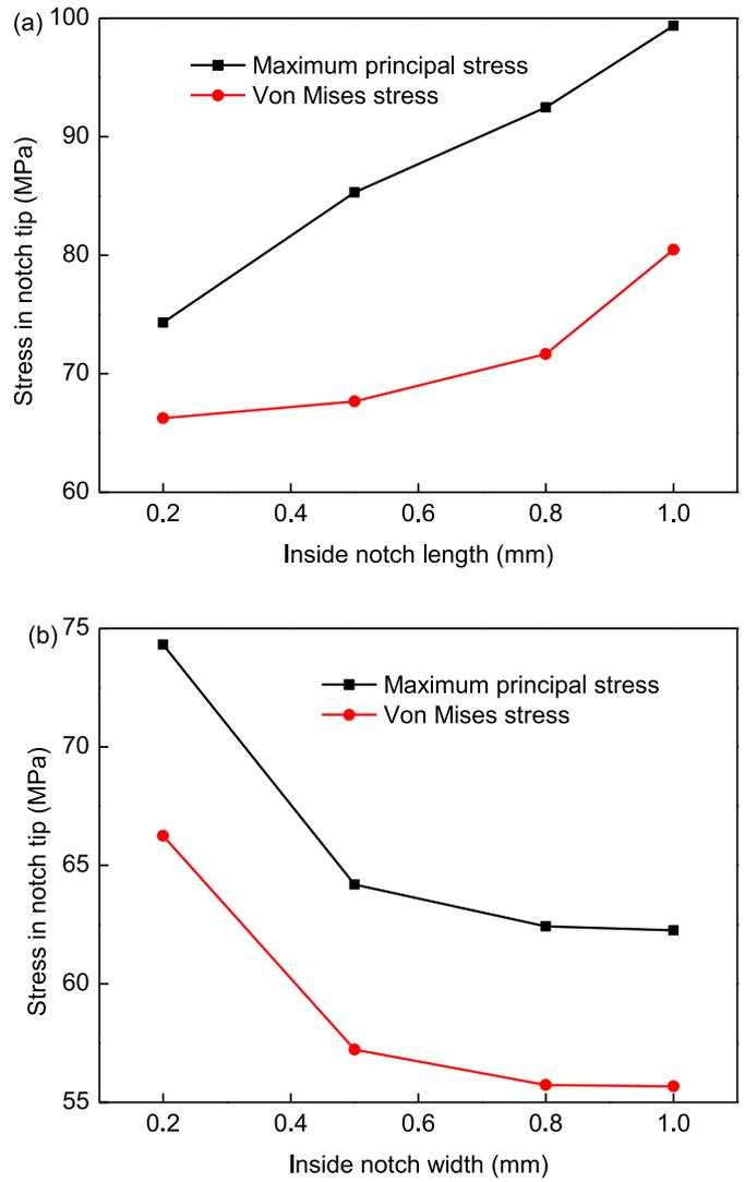
Fig. 17. Effects of notch length (a) and width (b) on maximum principal and Von Mises stress in notch tip.
