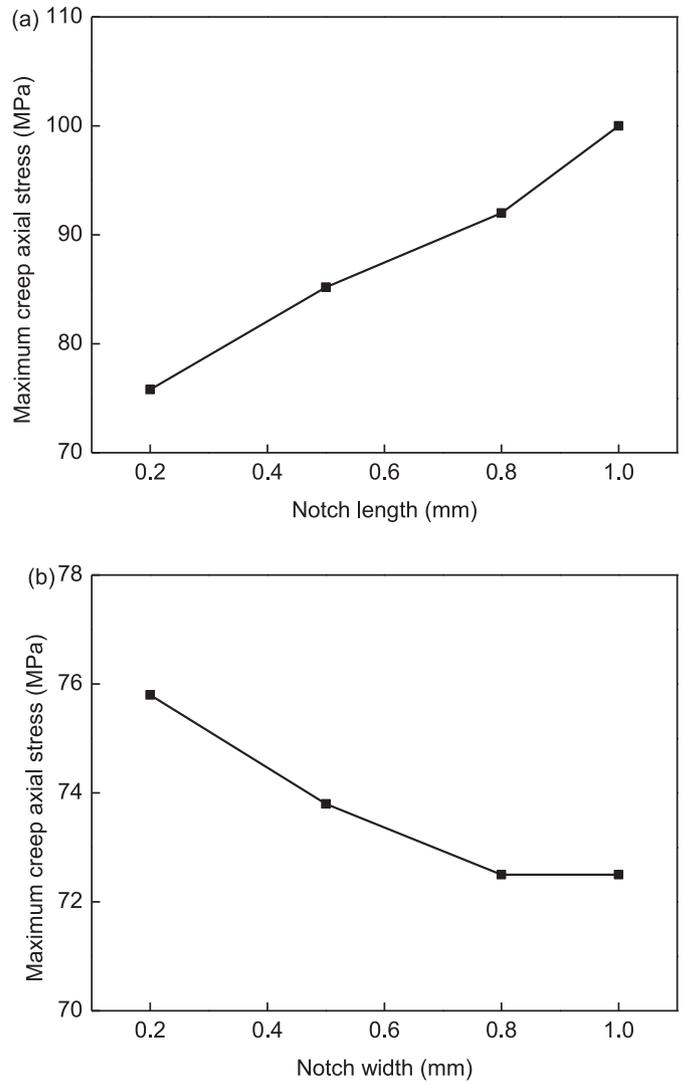
Fig. 14. The maximum creep axial stresses for inside notch with different notch lengths (a) and widths (b).
