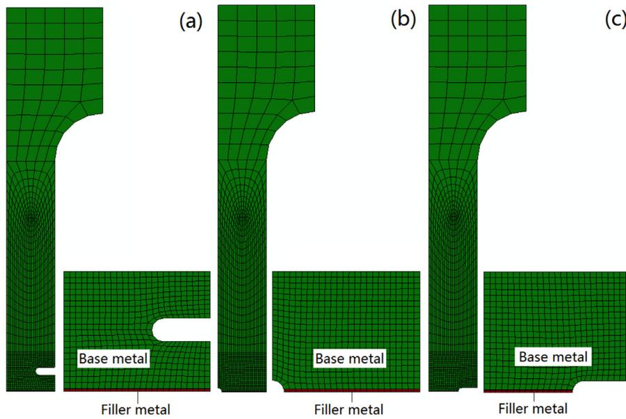
Fig. 2. Finite element meshing of (a) base notch, (b) inside notch and (c) surface notch.
