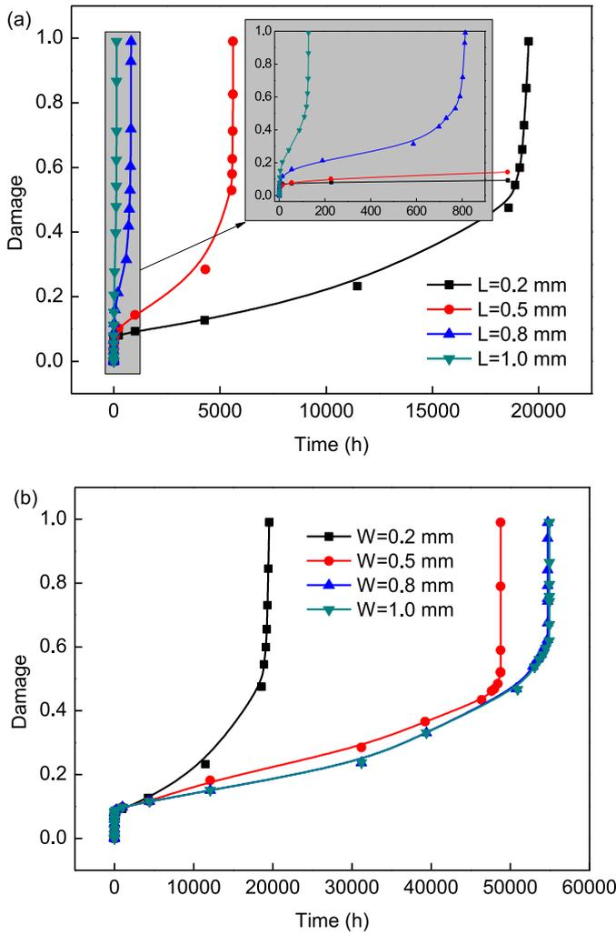
Fig. 13. Damage evolution with time for inside notch with different notch lengths (a) and widths (b).
