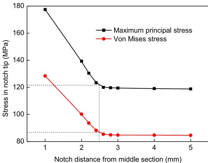
Fig. 16. The maximum principal and Von Mises stress in notch tip for base notch with different notch distances.
