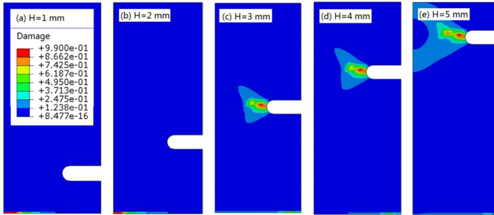
Fig. 7. Contours of creep damage for base notch with different notch distances.
