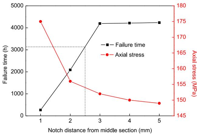
Fig. 10. The creep failure time and maximum creep axial stresses for base notch with different notch distances.
