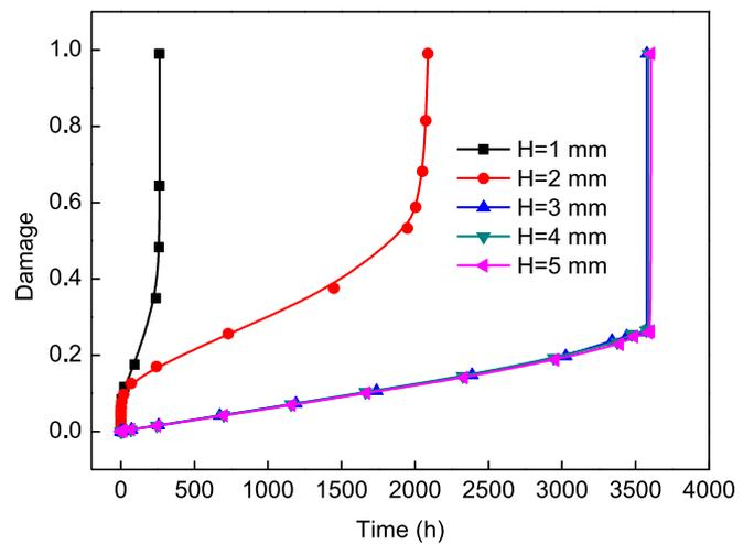
Fig. 9. Damage evolution with time for base notch with different notch distances.
