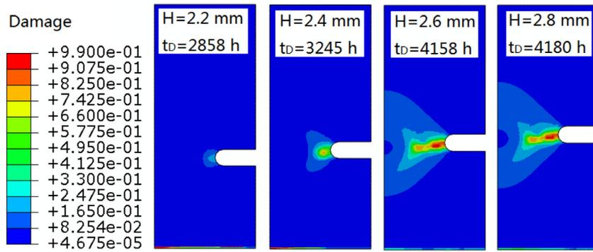
Fig. 11. Contours of creep damage for base notch with different notch distances.
