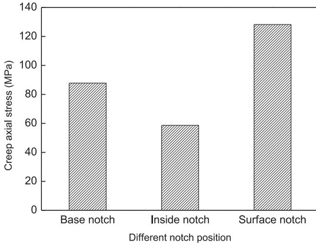
Fig. 5. The maximum creep axial stresses for different notch positions.
