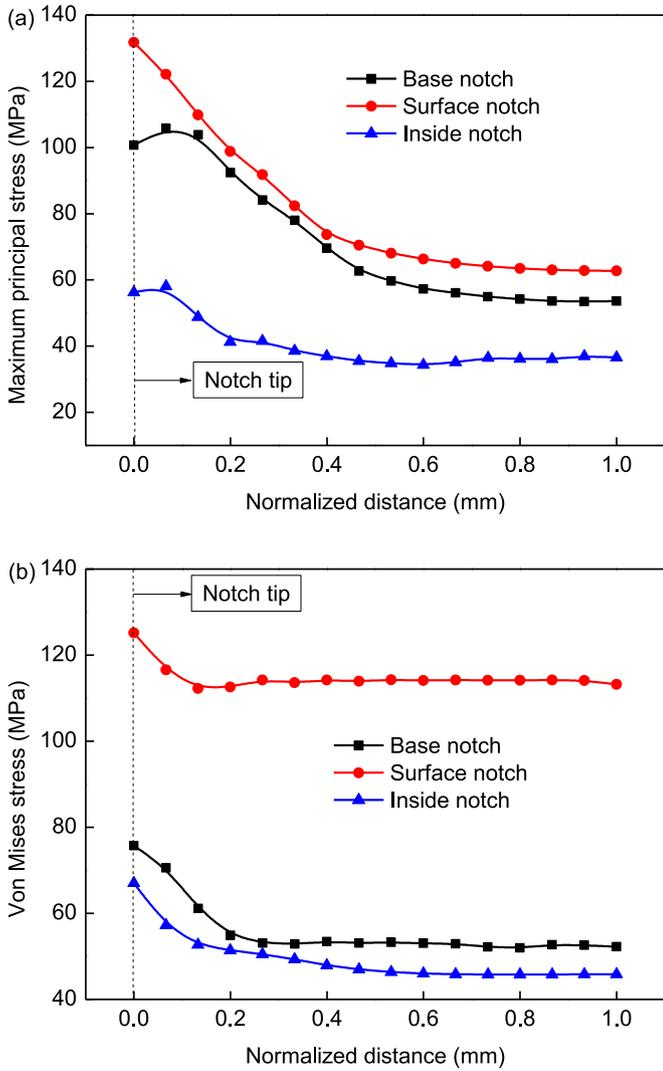
Fig. 15. The maximum principal stress (a) and Von Mises stress (b) along the normalized distance from notch tip for different notch positions.
