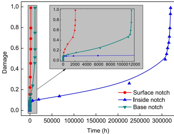
Fig. 4. Damage evolution with time for different notch positions.
