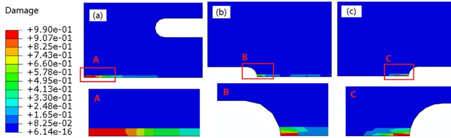
Fig. 3. Contours of creep damage of base notch (a), inside notch (b) and surface notch (c).
