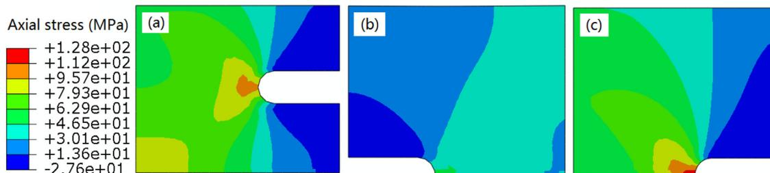
Fig. 6. The contour of creep axial stresses for base notch (a), inside notch (b) and surface notch (c).
