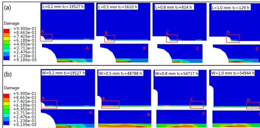
Fig. 12. Contours of creep damage for inside notch with different notch lengths (a) and widths (b).
