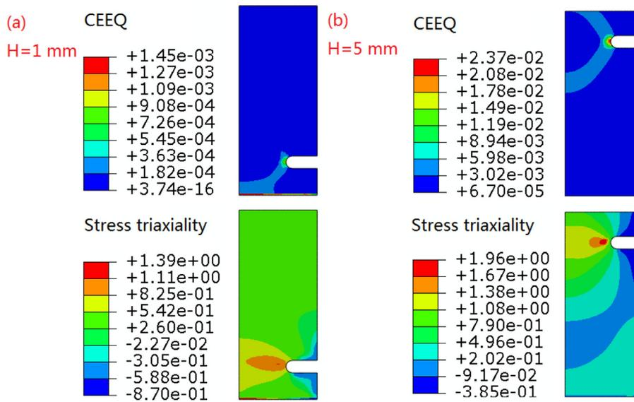
Fig. 8. Contours of CEEQ, stress triaxiality and micro-crack damage parameter for base notch with H = 1 (a) and 5 mm (b).
