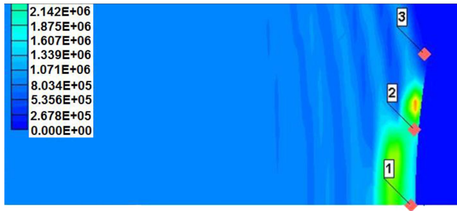
Fig. 14. Stress concentration at the point of first peak.
