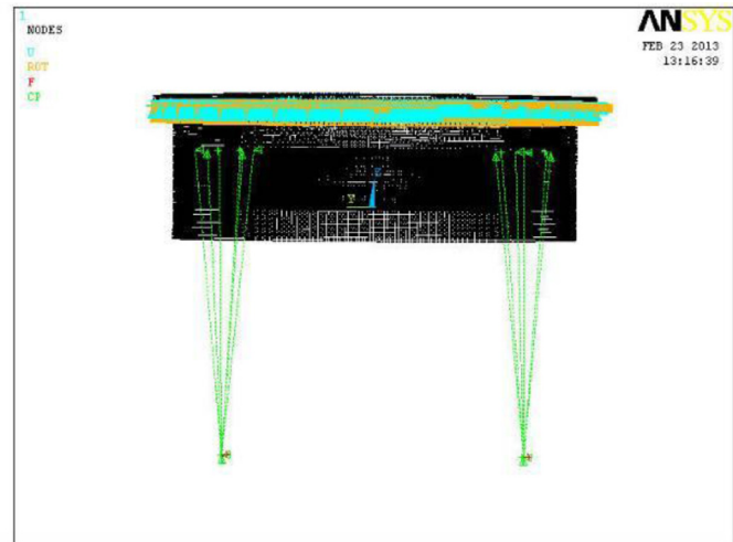
Fig. 11. Finite element model of the roof slab for harmonic analysis.
