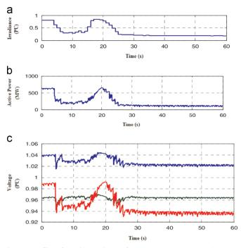
**Fig. 4.** The effect of variable irradiance of 10% PV penetration on irradiance (a), active power (b) and voltages (c) [20].
