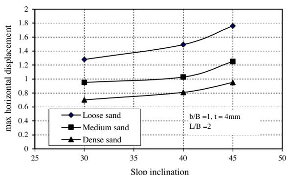
**Fig. 12** Maximum horizontal displacement versus slope inclination for monitoring points at different subgrade densities.
