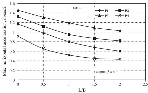
**Fig. 9** Maximum accelerations versus skirts ratio of monitoring points  $\gamma = 17 \text{ kN/m}^3$ .
