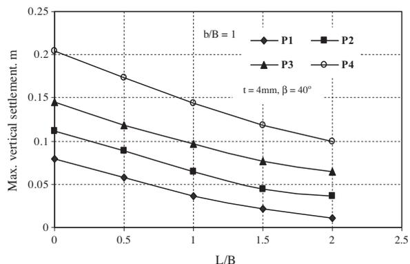
Fig. 6 Maximum vertical displacement versus skirts ratio of monitoring points  $\gamma = 17 \text{ kN/m}^3$ .
