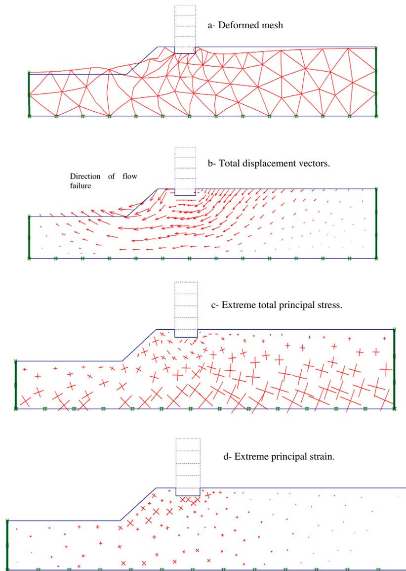
**Fig. 2** The finite element outputs of the non-skirted system  $\beta = 40^\circ$  and  $\gamma = 17 \text{ kN/m}^3$ .
