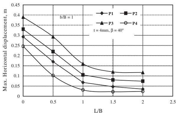
Fig. 5 Maximum horizontal displacement versus skirts ratio of monitoring points  $\gamma = 17 \text{ kN/m}^3$ .
