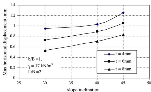
**Fig. 13** Maximum horizontal displacement versus slope inclination for monitoring point 3 at different skirt thicknesses.
