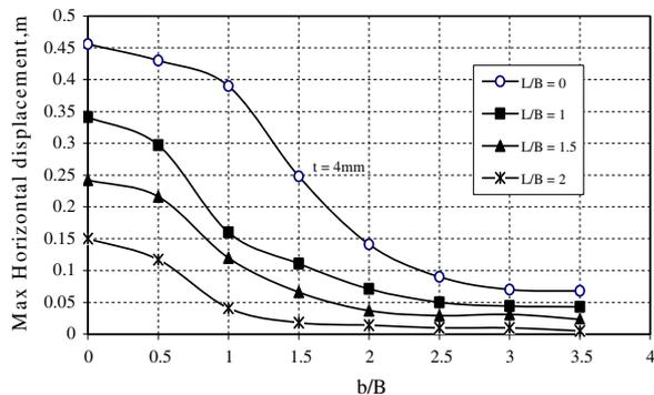
**Fig. 10** Maximum horizontal displacement versus distance from slope crest for monitoring points 3 at the slope toe  $\gamma = 17 \text{ kN/m}^3$ .
