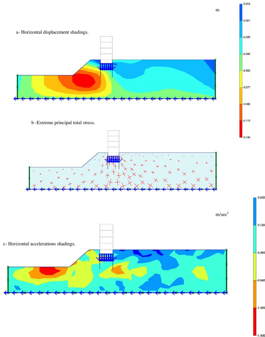
**Fig. 3** The finite element outputs of the skirted system at  $L/B = 1$ ,  $b/B = 1$   $t = 4$  mm,  $\beta = 40^\circ$  and  $\gamma = 17$  kN/m<sup>3</sup>.
