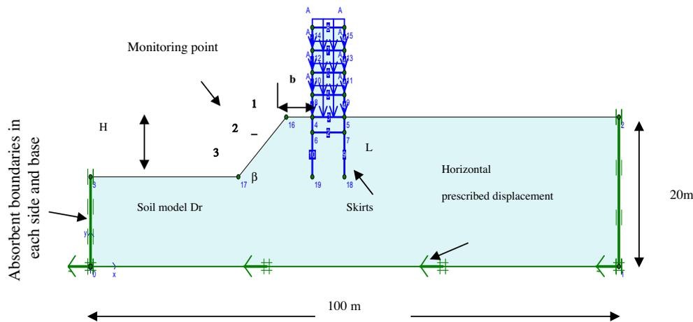
Fig. 1 The geometry of the finite element model and studied parameters.
