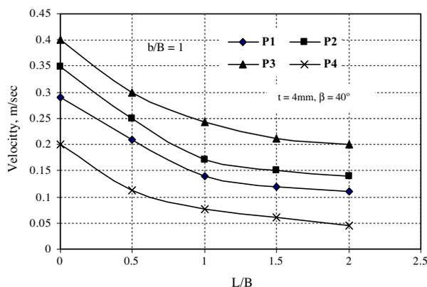
Fig. 8 Maximum velocity versus skirts ratio of monitoring points  $\gamma = 17 \text{ kN/m}^3$ .
