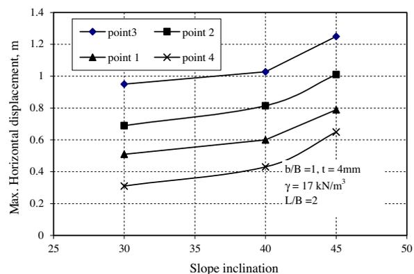
**Fig. 11** Maximum horizontal displacement versus slope inclination for monitoring points.
