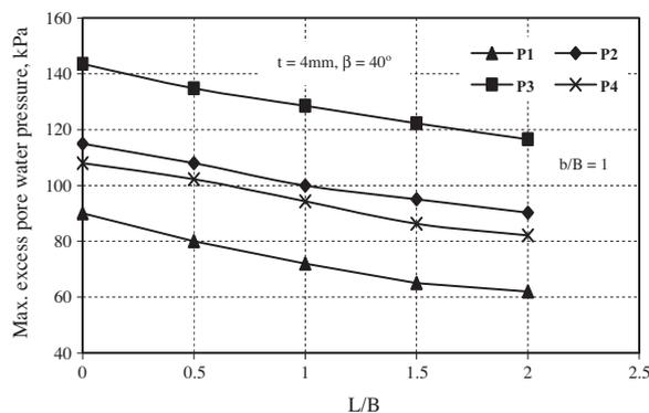
Fig. 7 Maximum excess pore water pressure versus skirts ratio of monitoring points  $\gamma = 17 \text{ kN/m}^3$ .
