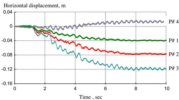
**Fig. 4** Horizontal displacement time history for slope during earthquake.  $L/B = 2$ ,  $b/B = 1$  m  $t = 4$  mm,  $\beta = 40^\circ$  and  $\gamma = 17$  kN/m<sup>3</sup>.
