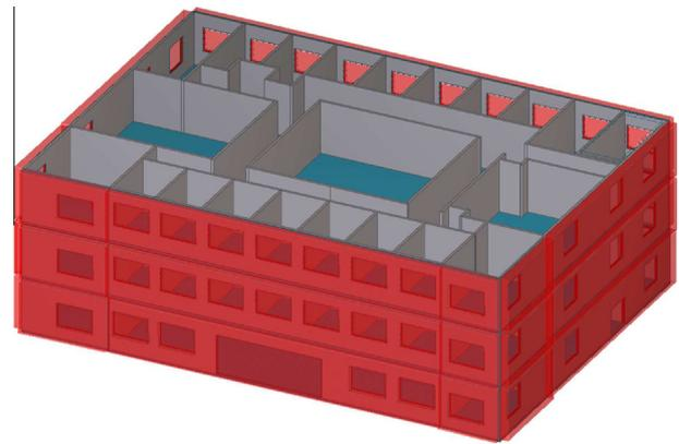
Fig. 18. Exterior work packages detected around the building perimeter.
