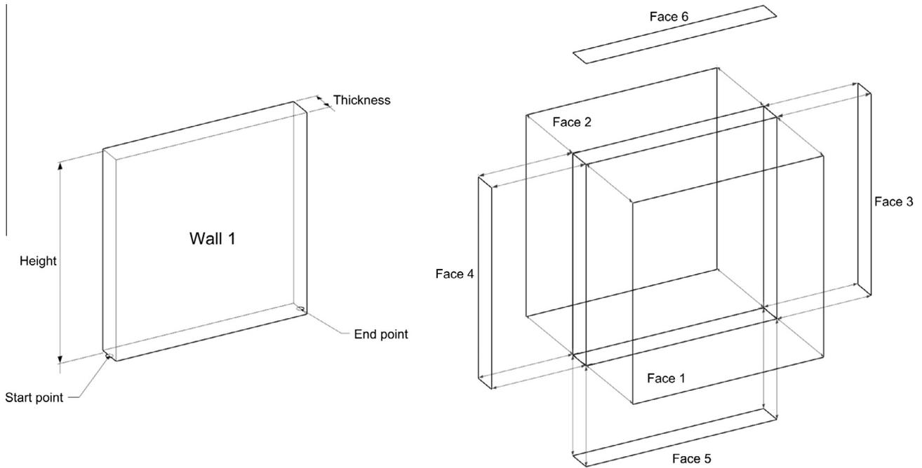
Fig. 1. A wall component (a) and its decomposition into face objects (b).
