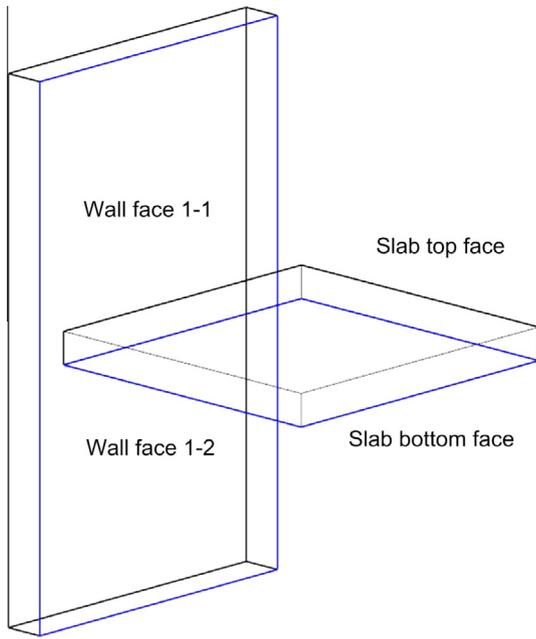
Fig. 4. A slab bottom face as the middle face of a wall face.
