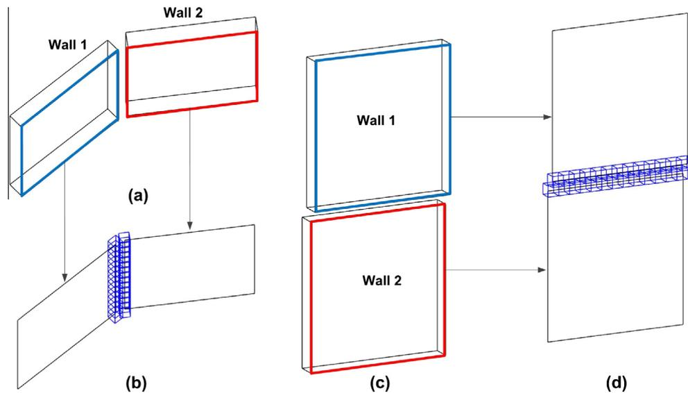
Fig. 7. Adjacency assessment based on cell collision.
