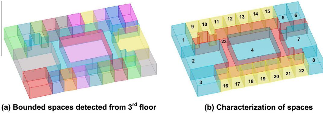
Fig. 19. Detection and characterization of bounded spaces from 3rd floor.
