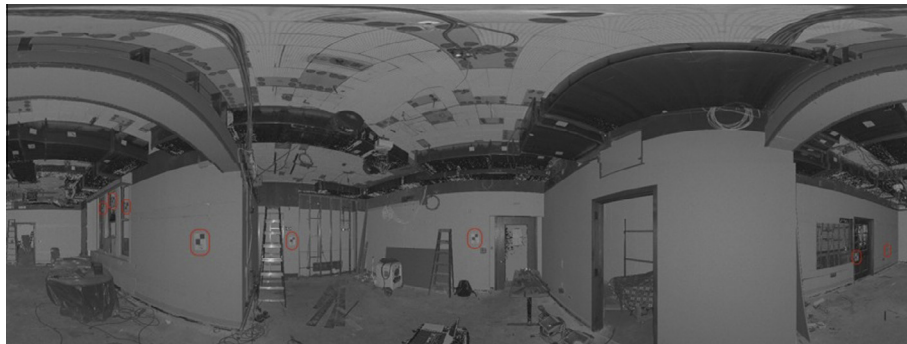
Fig. 2. Targets shown in a point cloud.
