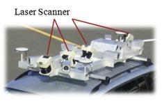
**Fig. 1.** Mobile mapping system [14].
