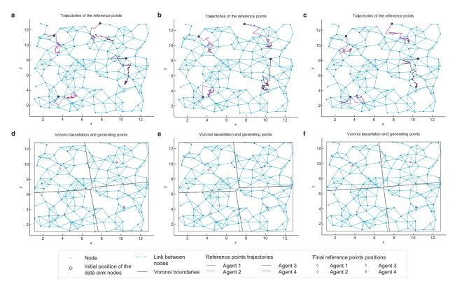
**Fig. 2.** Simulation 2, upper plots: trajectories of the generating points until time-step h = 200: (a) uniform metric, (b) node degree metric, (c) leftover energy metric. Lower plots: reference points and Voronoi regions at the end of the simulation: (d) uniform metric, (e) node degree metric, (f) leftover energy metric.
