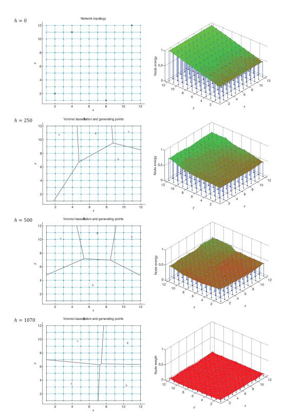
**Fig. 4.** Simulation 4, left plots: reference points of the data sink nodes and Voronoi regions during the simulation, right plots: leftover node energy during the simulation. In the figure, the node energy level is represented by a bar on the *z*-axis starting from the node position on the (x, y) plane; the figure also shows an envelope plane for presentation clarity.
