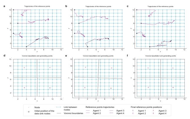
**Fig. 1.** Simulation 1, upper plots: trajectories of the generating points until time-step h = 200: (a) uniform metric, (b) node degree metric, (c) leftover energy metric. Lower plots: reference points and Voronoi regions at the end of the simulation: (d) uniform metric, (e) node degree metric, (f) leftover made energy metric.
