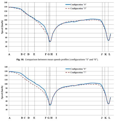
Fig. 11. Comparison between mean speeds profiles (configurations "7" and "0").
