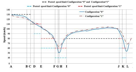
Fig. 7. Comparison between mean speed profiles (configurations "1" and "0").
