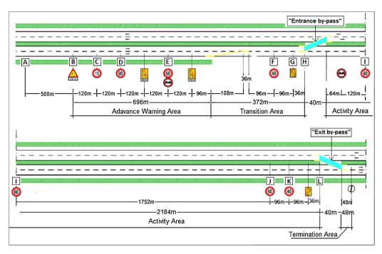
Fig. 5. Speed measurement sites (configuration "0").
