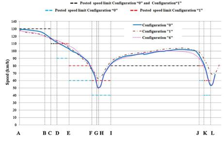
Fig. 8. Comparison between mean speed profiles (configurations "0", "1" and "6").
