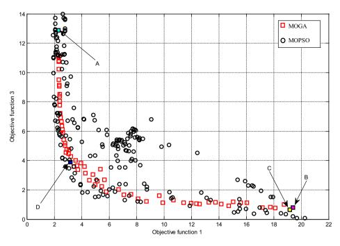
Fig. 18. Pareto fronts of objective functions 1 and 3 for the inverted pendulum system.
