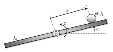
Fig. 1. Structure of the ball-beam system.
