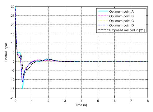
Fig. 11. Time response of the driving force for the ball-beam system.
