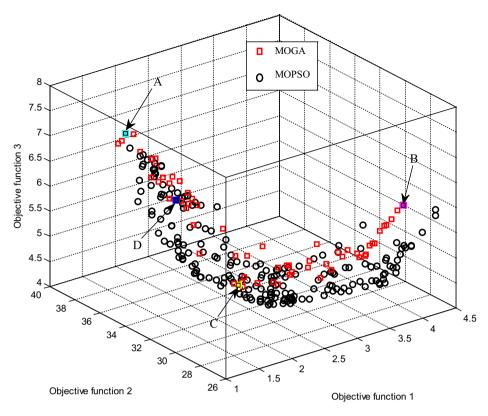
Fig. 5. Three-dimensional Pareto fronts of objective functions 1, 2 and 3 for the ball-beam system.
