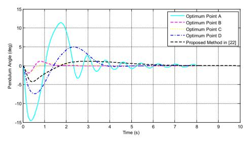
Fig. 21. Time response of the pendulum angle for the inverted pendulum system.
