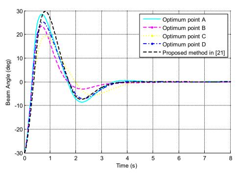
Fig. 10. Time response of the beam angle for the ball-beam system.
