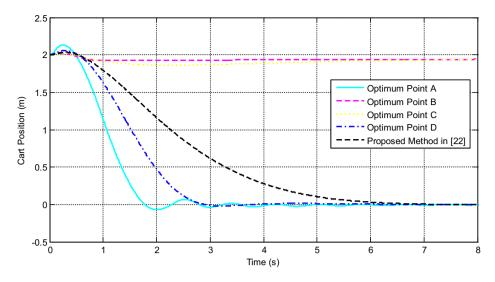
Fig. 20. Time response of the cart position for the inverted pendulum system.
