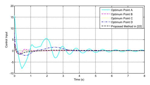
$\textbf{Fig. 22.} \ \ \text{Time response of the driving force for the inverted pendulum system}.$
