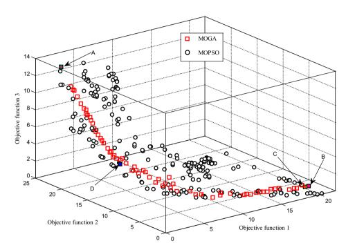
Fig. 16. Three-dimensional Pareto fronts of objective functions 1, 2 and 3 for the inverted pendulum system.
