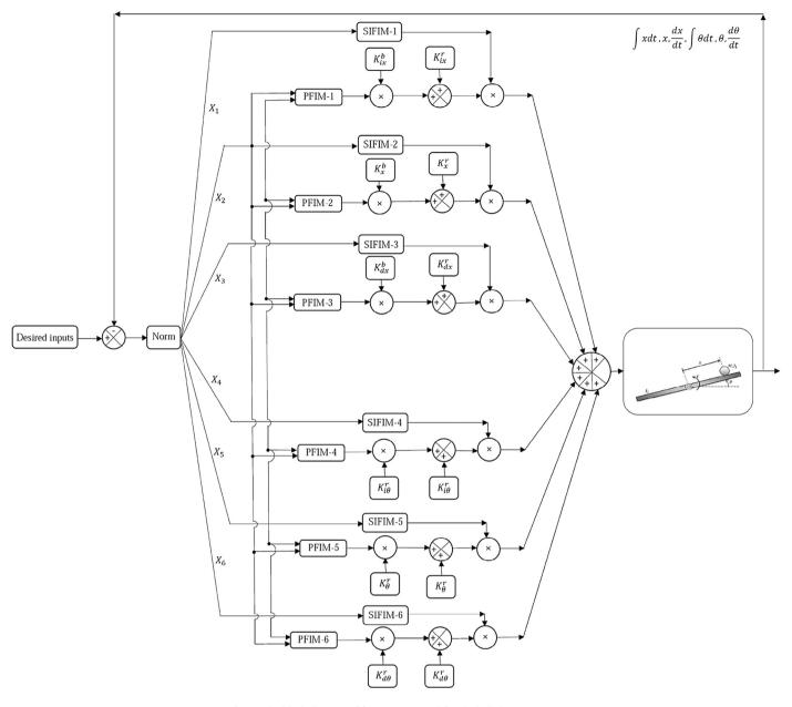
$\textbf{Fig. 2.} \ \ \textbf{The block diagram of fuzzy-PID control for the ball-beam system}.$
