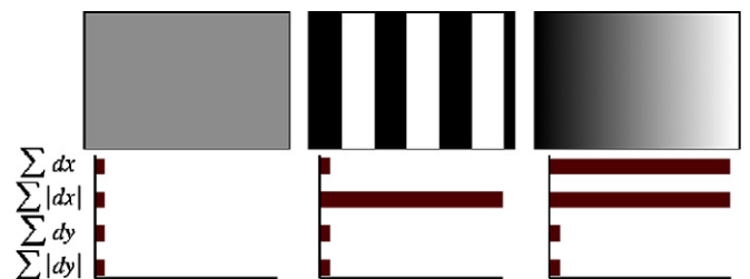
Fig. 13. The descriptor entries of a sub-region represent the nature of the underlying intensity pattern. Left: In case of a homogeneous region, all values are relatively low. Middle: In presence of frequencies in x direction, the value of \sum |d_x| is high, but all others remain low. If the intensity is gradually increasing in x direction, both values \sum d_x and \sum |d_x| are high.
