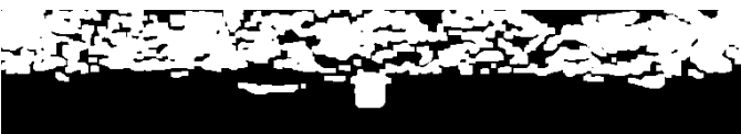
Fig. 8: Black and white image of the Obstacle map after post-processing. The small holes in Figure 7 are filled.
