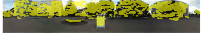
Fig. 9: Original lower image with obstacles overlaid on it. The pixels in yellow correspond to obstacles.
