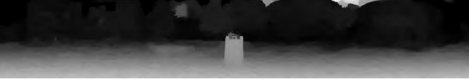
Fig. 4: Disparity map generated from optical flow estimation. Brighter pixels correspond to greater disparity and so smaller depth. We observe uniform gradient of disparity along the ground plane, in the bottom half of the image.
