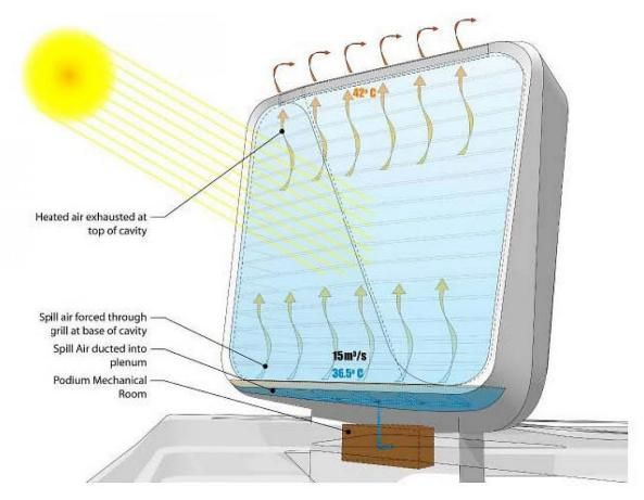
As mentioned above air rom the podium HVAC system is 'spilled' into the DSF. This is another subtle innovation: that the DSF is just a fancy exhaust plenum for the podiums.
