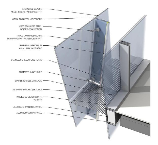
The inner layer of the DSF is a simple curtain wall. The only eccentricity is that the panels are designed to the angles of each tower's facade. In fact, the glazing of the inner layer has a very low level of solar radiation protection. To meet the Estidama requirements this coating is not required, but it does provide some additional comfort and reduces the reflectivity of the glass.
