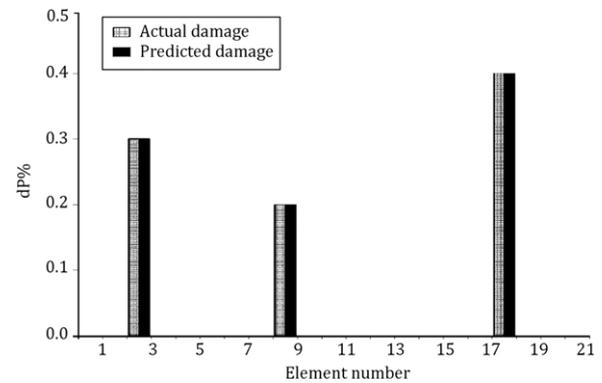
Figure 10: Predicted damage of frame, Scenario 3 (noise free data).
