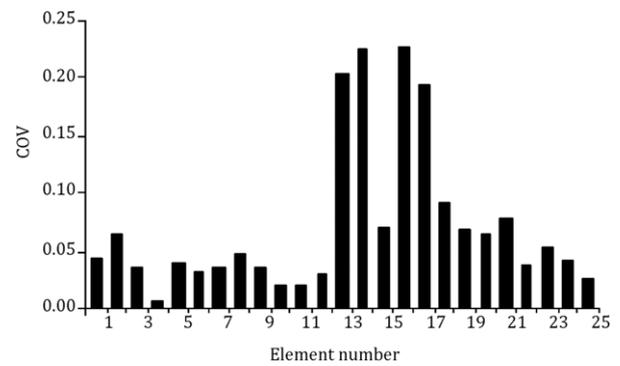
Figure 20: Example of the standard deviation of predicted parameters of a truss identification case.
