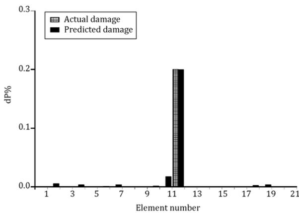
Figure 17: Predicted damage of frame, Scenario 2 (noisy data).
