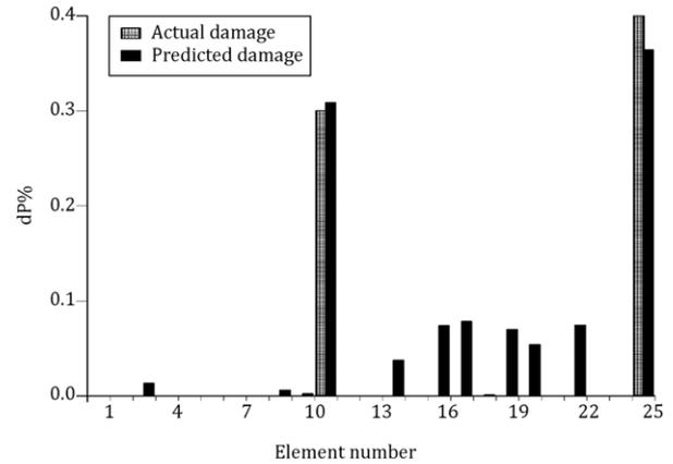
Figure 13: Predicted damage of truss, Scenario 2 (noisy data).
