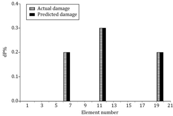
Figure 11: Predicted damage of frame, Scenario 4 (noise free data).
