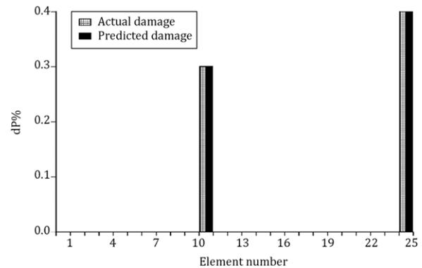
Figure 4: Predicted damage of truss, Scenario 2 (noise free data).
