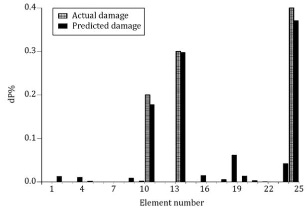
Figure 15: Predicted damage of truss, Scenario 4 (noisy data).
