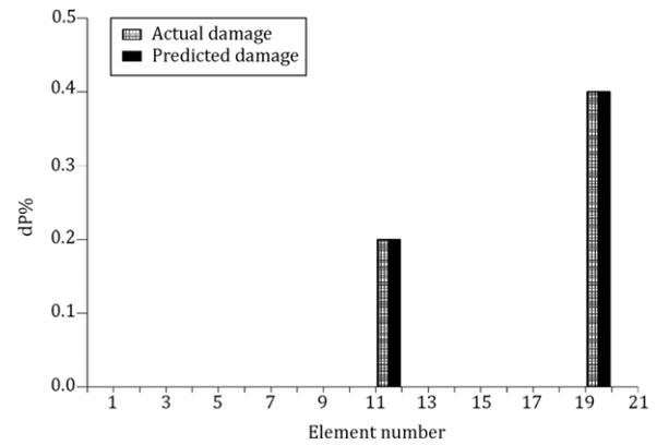
Figure 8: Predicted damage of frame, Scenario 1 (noise free data).
