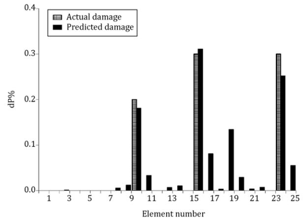
Figure 14: Predicted damage of truss, Scenario 3 (noisy data).
