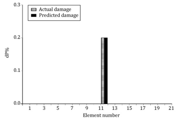
Figure 9: Predicted damage of frame, Scenario 2 (noise free data).
