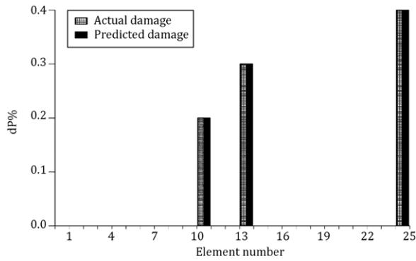
Figure 5: Predicted damage of truss, Scenario 3 (noise free data).
