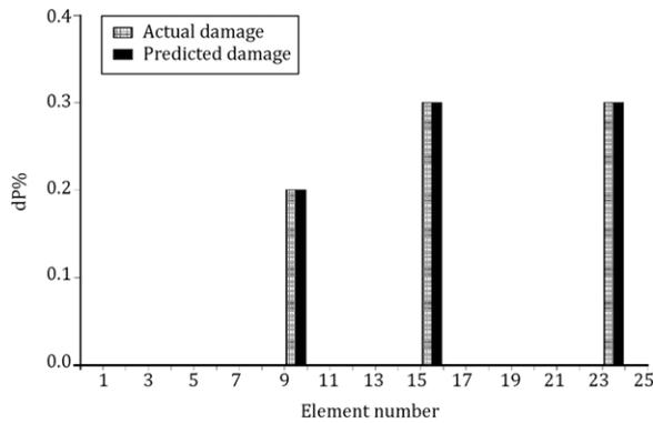
Figure 6: Predicted damage of truss, Scenario 4 (noise free data).
