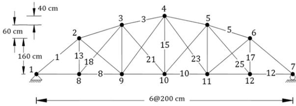
Figure 1: Geometry of bowstring truss.
