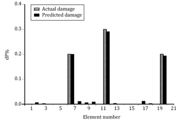
Figure 19: Predicted damage of frame, Scenario 4 (noisy free data).
