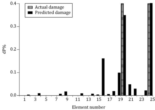
Figure 12: Predicted damage of truss, Scenario 1 (noisy data).
