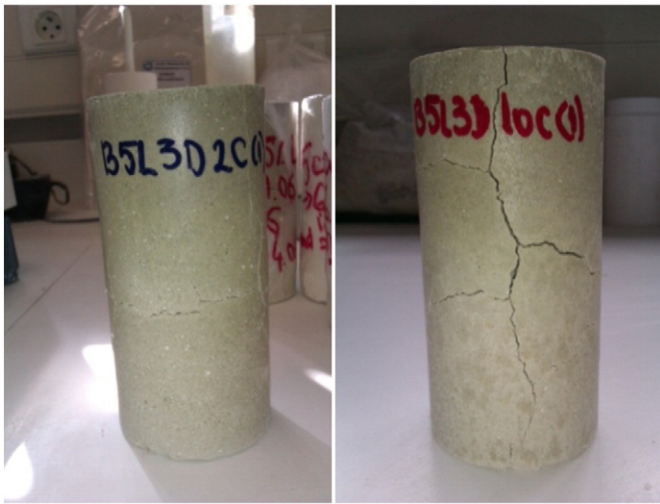
Fig. 3. Treated bentonite samples, cured for 3 days and subjected to 2 (left) and 10 (right) freeze–thaw cycles.
