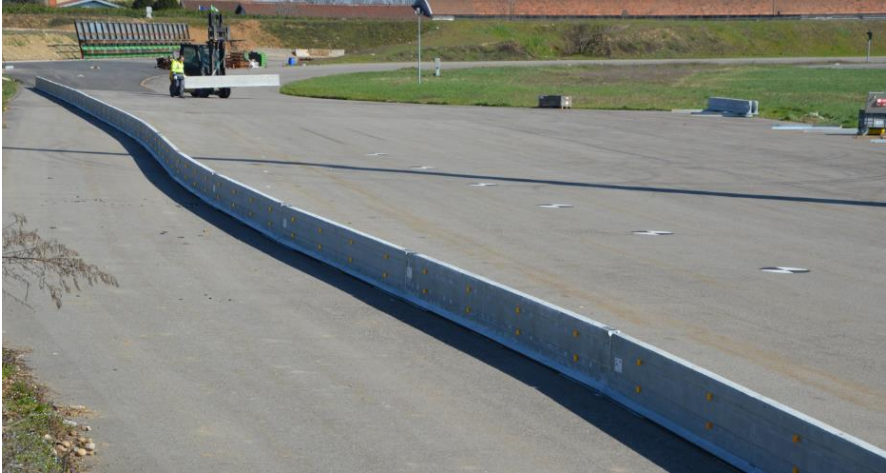
FIGURE 5 Working width W2 after a TB41/T3 impact (36,6kJ impact energy) on a 125kg/m slim-type barrier
