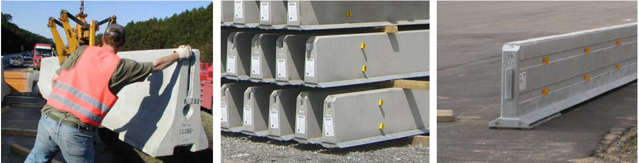
FIGURE 5 Standard New Jersey type barriers at 500kg/m, 60cm width (l), slim type barriers at 180kg/m, 32cm width (m), superlight slim-type barriers at 125kg/m, 24 cm width (r)
