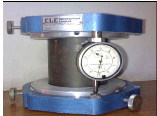
Figure-2. Device used to obtain stress-strain relationship.
