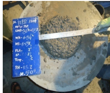
Figure 10. Flow Test of Trial HPC Mix
