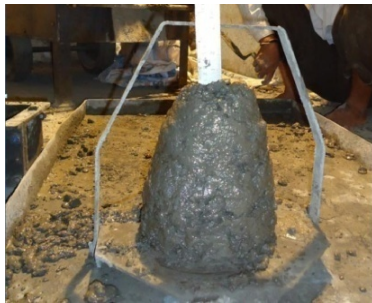
Figure 9. Slump Test of Trial HPC
