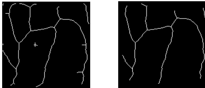
Fig. 5. Left: Skeleton of the vein pattern in Figure 4; Right: After pruning
