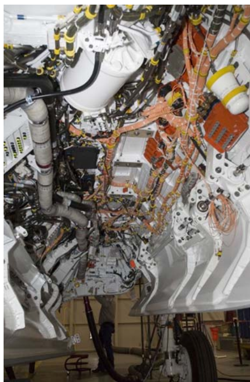
Fig. 1 Example electrical wiring and pipe loom in weapons bay of F-35 JSF [5]
