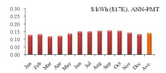
Fig. 7 PV Electricity cost, \$17K, mortgage: 1%
