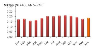
Fig. 5 PV Electricity cost, \$14K, mortgage: 6%
