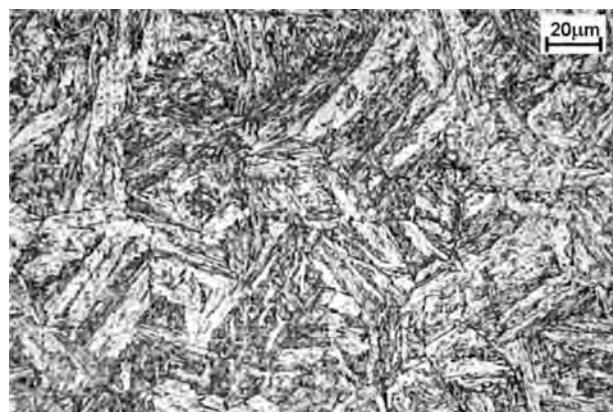
Fig. 1. Microstructure of the base metal after welding; martensitic microstructure
